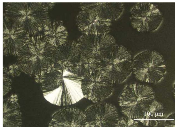
Figure 3. The morphology of dark and bright spherulites of PVDF after isothermal crystallization for 4 h at 160 °C. [Color figure can be viewed in the online issue, which is available at wileyonlinelibrary.com .]
